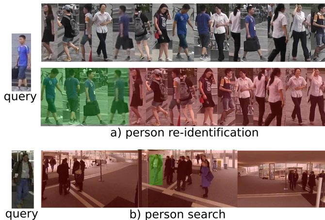
Fig. 1: Demonstration of the search process for one gallery image for the person re-identification (a), and person search (b), problems. The red boxes indicate the wrong matched results while the green box represents the truly matched person.
